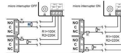
The relays can be used to act on any type of electrical circuit, being able to act in an NA or NC way depending on the terminals used. Verify in the Technical Features section the current and maximum voltage value of relay contacts.
